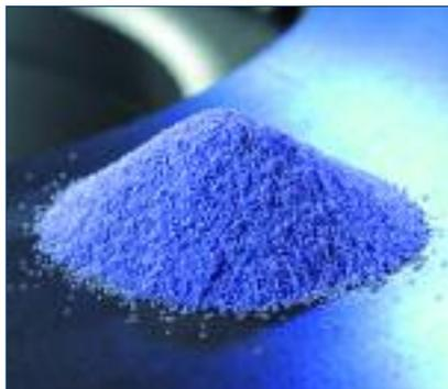
Microcrystalline sintered alumina
